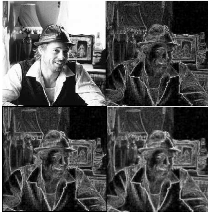
Figure 6. Haantjes-Finsler curvature of an image with respect to different scales. From top left in clockwise direction: original image, 3X3, 7X7 and 5X5 window size.
